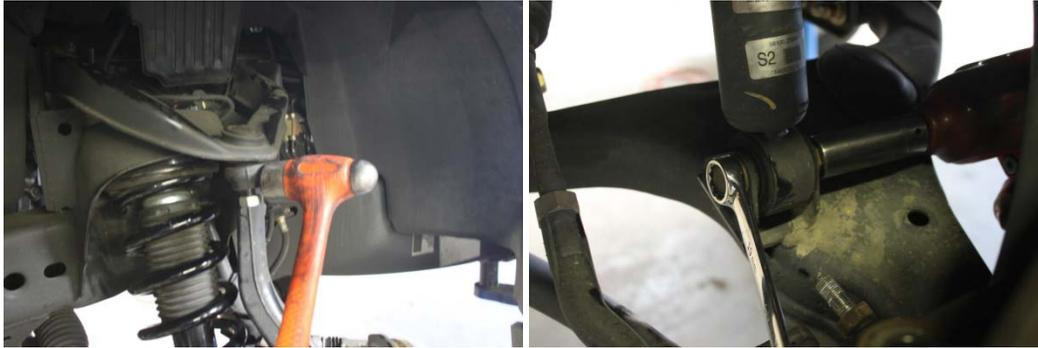
4) Remove the strut from the vehicle and mount it in a bench vise, and install the strut spacer kit. Torque fasteners to OEM specification. **Note the shape of the spacer, the strut will be rotated 180 degrees when installed.**
